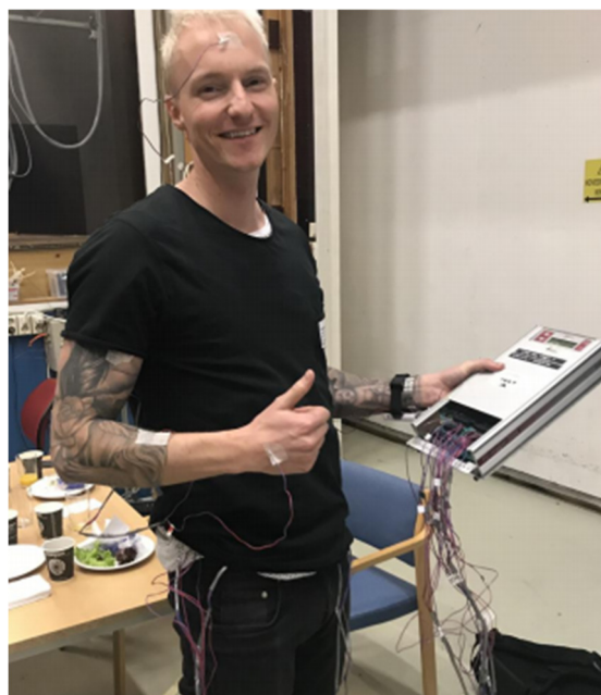
Figure 3. Measurements of skin temperatures in SvalVent are important for better understanding of the effect of cooling air speed on comfort and satisfaction. Photo: SINTEF
