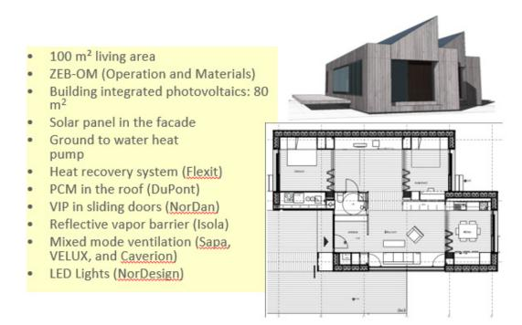
Figure 1. The design and technology included in ZEB living lab, Illustration NTNU
