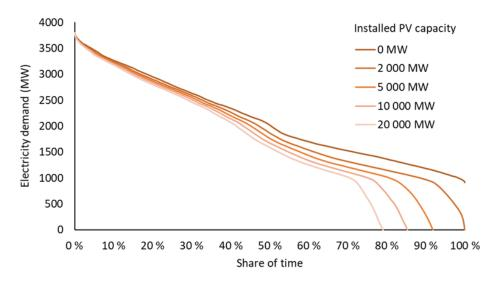
Figure 6.1: Load duration curve of the electricity demand in the region of Oslo with different levels of PV capacity
