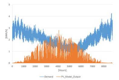
Figure 4.1: Load curve for typical residential customer and modelled PV generation [39]
