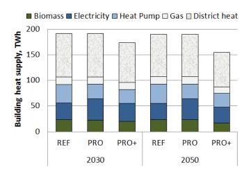
Figure 6.4: Heat supplied to buildings by different types of technology for all cases in 2030 and 2050
