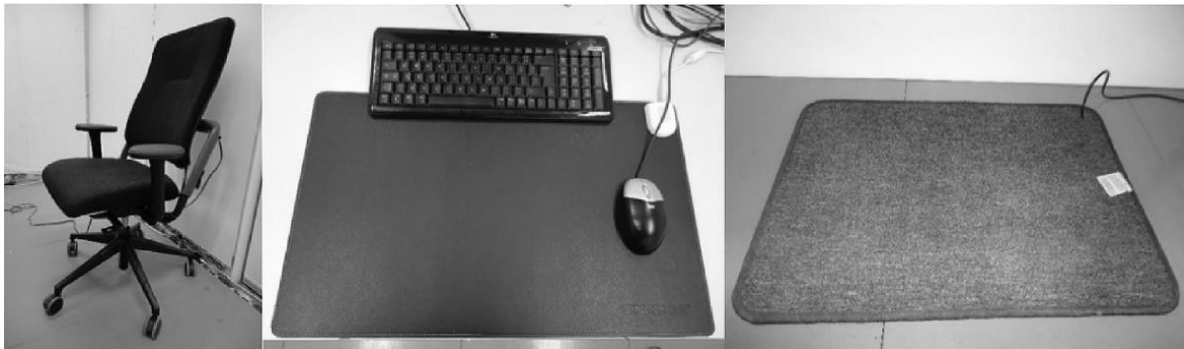
Figure 10 Tested personalized heating system: heated chair (left), heated desk mat (middle) and heated floor mat (right). (Vesely et al. 2017: page 224) https://creativecommons.org/licenses/by/4.0/
