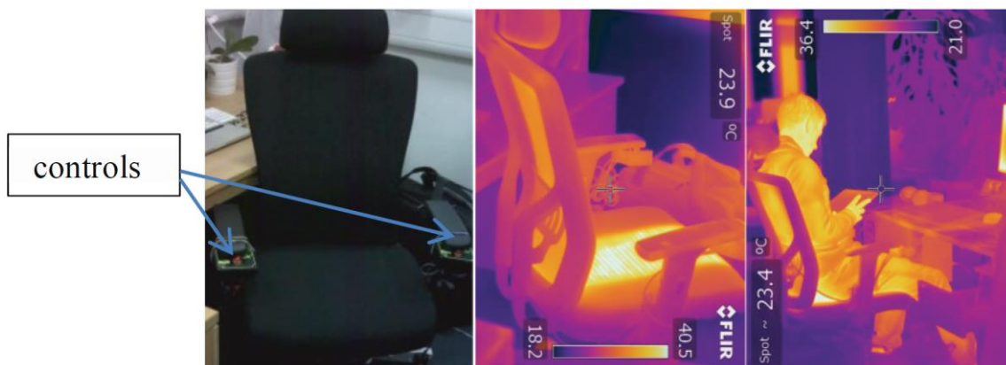
Figure 11 Thermal chair: design (left), thermal image of seat temp (FLIR T660) (middle) and in use (right). (Shahzad, Hughes, et al. 2017: page 2636)
